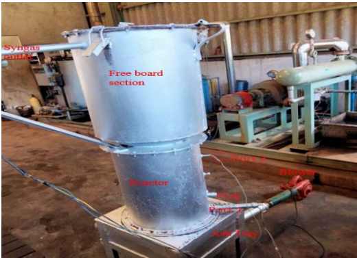
Figure 3. Fixed bed gasifier at JKUAT showing port 1 and 2 (Fernando, 2014; Nduku Nzove, 2021)
