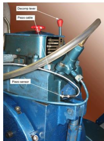
Figure 7. Piezo sensor to measure in cylinder pressure
