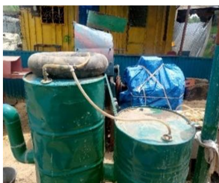
Figure 7. Measuring biogas volume using an air chamber
