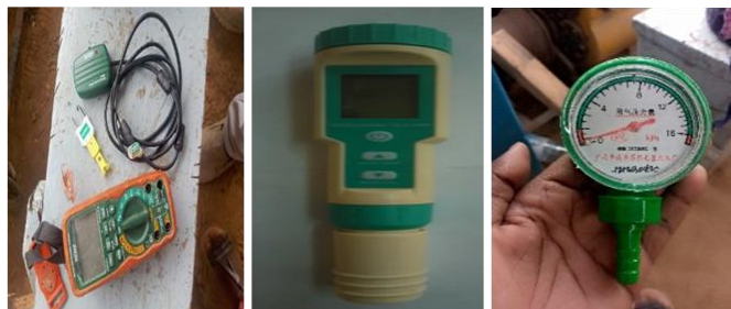
Figure 4. Temperature sensor (a), pH meter model C-600 (b), pressure gauge (c)
