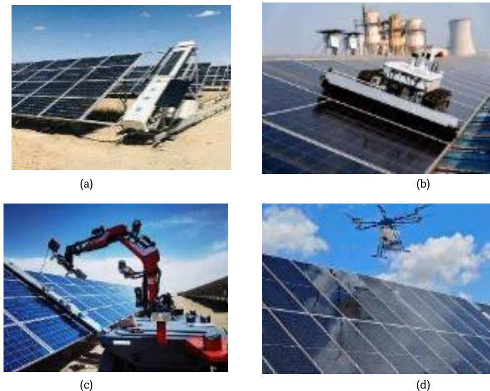
Figure 3. (a) Rail-Mounted PV Cleaning Robot (b) Tracked PV Cleaning Robot, c. UAV-Integrated Cleaning Robot, d. AGV-Based Brush Cleaning Robot
